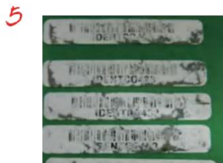
Spatter or direct contact with soldering flux label damage
