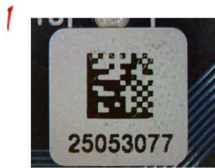
The high temperature label blurring and bubbling
